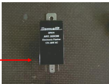
Direction light generator unit
